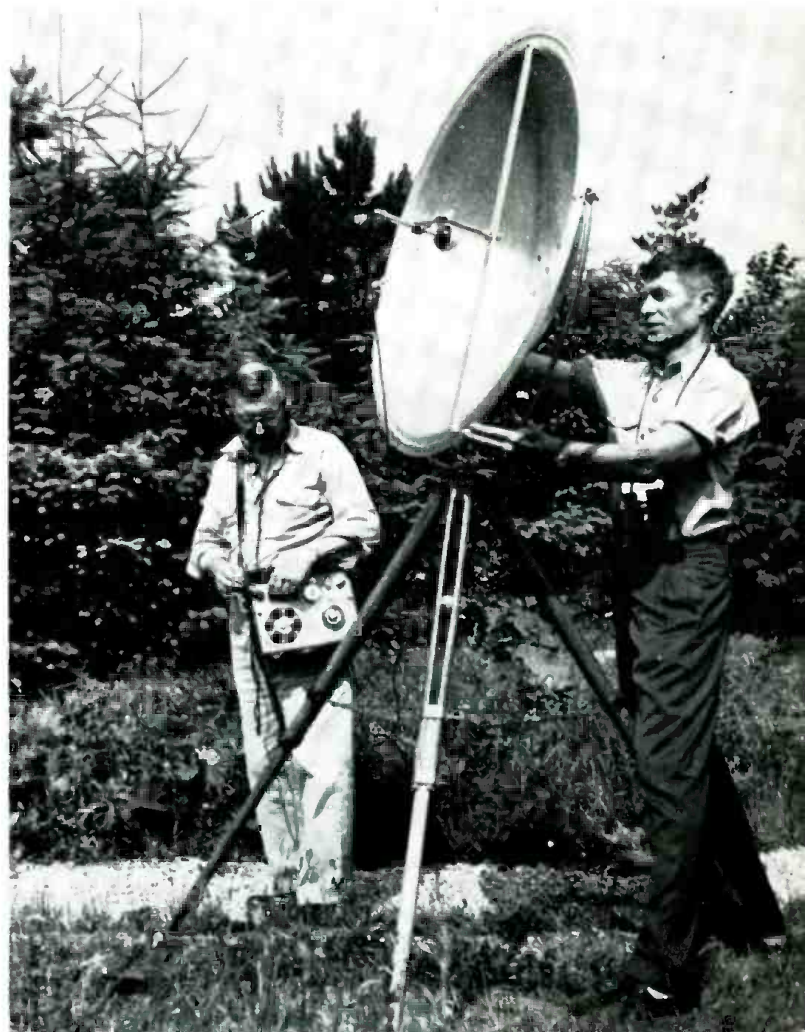
The author (right), and Dr. Carl R. Reese, a colleague, capture a bird's melody with a Magnemite portable, and microphone mounted in a 40 inch parabolic reflector. The parabola is aimed by sighting through a small hole near the center.
