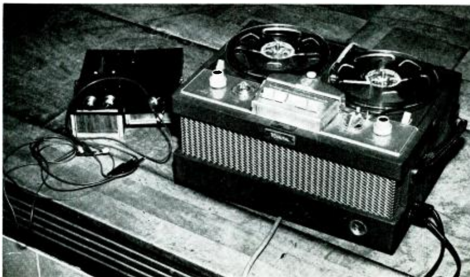
A VM binaural tape recorder and accessories. Beside the recorder is a dual corded Telex monitor set, and microphone case. A case for your mikes is a good investment.
