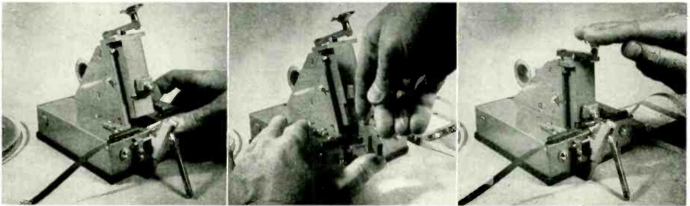
The Reiter Skila splicer automatically applies splicing tape and trims splice. The tape is positioned in the guides and rubber rollers hold it in place. The cutter bar assembly is raised and the handle pushed away or pulled toward the operator to cut tape. A carboly wheel makes the cut. Chip is removed and the knob on top pressed. This ejects tape, applies it and trims splice all in one operation.
