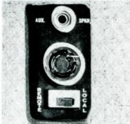
Upper: remote control switch turns on or off and in second position turns on playback or record. Lower: Rear of case has auxiliary speaker jack, socket for remote control cord and local-remote control switch.
